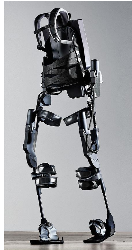
A medical prosthetic-style exoskeleton to help paralyzed people walk. Source: http://wonderfuleengineering.com
